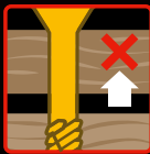
Partially Threaded Stops The Timber Jacking
