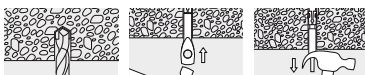
Drill required diameter hole Lightly tap the anchor into the hole Set anchor using a claw hammer
